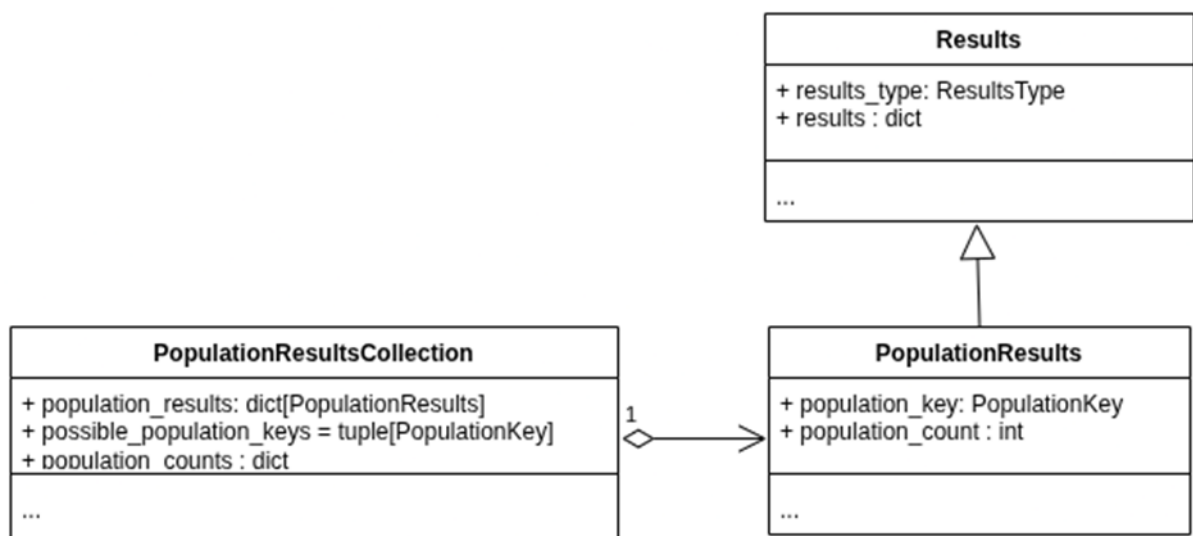
Figure 47: Simplified UML diagram showing the working principle of PopulationResultsCollection
